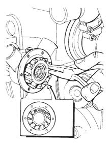
Check the impeller. The impeller can be damaged, mostly because of lack of water in the pump due to blocked intake or because of inproper winter storage.
