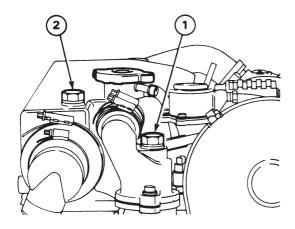
**The sea-water system.** Close the sea-water cock. Loosen both the hose connections from the sea-water pump and seawater filter (optional) at the reverse gear/S-drive and point them downwards so that the water runs out.
