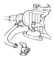
Loosen the hose between the sea-water intake and the reverse gear/S-drive. Connect a hose and put the other end in a bucket with fresh water. Provide for the topping-up of fresh water into the bucket. Run the engine at fast idle a few minutes.
