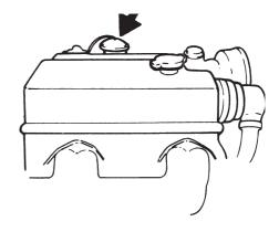
Check the engine oil level. This should be within the area marked on the dipstick. Fill with oil when necessary through the oil filler.
