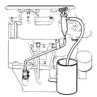
Pump out all oil from the engine and reverse gear. Use an oil suction pump or electric type pump designed for this job.
