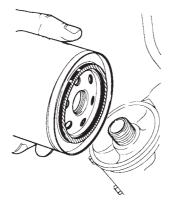
Change the oil filter. The oil filter is to be changed the first time after 20 hours of operation and then after every 200 hours of operation. Screw off the old filter. If the oil filter is difficult to unscrew, there is a special tool which can be used.
