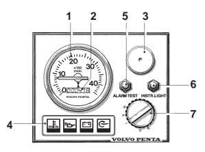
Instrument panel (standard)\* with key switch \*Note. Rev. counter with built-in hour counter is optional.
