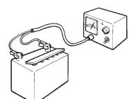
Remove the batteries from the boat. Clean them and store them in a cool, dry place. Check that the batteries are well charged. Trickle charge them according to the manufacturer's instructions (a flat battery can easily be damaged as a result of freezing).
