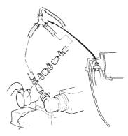
If the engine has a vacuum valve it must be taken apart twice a season or whenever leaks occur.
