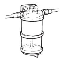
Change the insert in any extra fuel filter fitted. Close the fuel cocks at the tank. Be careful not to spill fuel!
