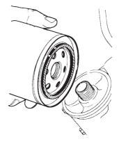
Change the oil filter.\* If the engine is fitted with an S-drive this should be drained when the boat is laid up. Fill up the engine and reverse gear to the correct level with Volvo Penta diesel engine oil\*, which also has corrosion protective properties. Start the engine and check for leaks. The engine is now ready to run on this oil next season.
