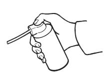
Clean the outside of engine, and reverse gear/Sdrive. Touch-up any bare patches in the paintwork with Volvo Penta original paint. Spray the components of the electrical system, and all the control components with anti-moisture spray. All engine control linkages should be inspected for wear, properly adjusted and protected from corrosion.
