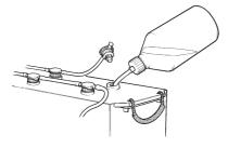
Check the level of electrolyte in the battery (batteries). The level should be 5–10 mm (3/16"–3/8") above the cell plates in the battery. If necessary, topup with distilled water.
