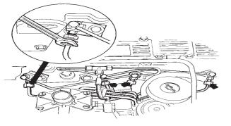
Loosen the fuel pressure pipe nuts at the injectors and set the speed control to full speed. Turn the engine at full starter motor speed until fuel flows from the fuel pressure pipes. Watch out for fuel spillage. Use rags or similar around the venting screw. Tighten the fuel pressure pipe nuts and start the engine.
