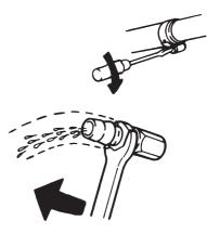
Check the tightening of all hose-clamps. Check that all drain-cocks are closed and tight. Clean the engine and reverse gear on the outside. Check the exhausthoses. Install the impeller.
