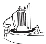
In boats fitted with S-drive, the rubber seal between the drive and the bedding should be checked carefully. **The seal should be changed every seven years.** This should be done by an authorized Volvo Penta dealer.
