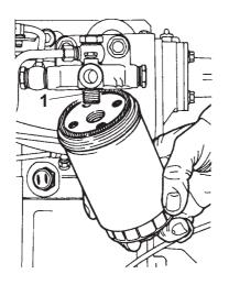
Change the fuel filter. Unscrew the fuel filter using a filter remover or other suitable tool. Ensure that the nipple (1) is firmly seated in the filter head. Screw on the new filter and tighten by hand. Vent the system, start the engine and check for any leakage
