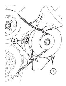
Repace the v-belt. Loosen the alternator mounting bolts 1 and 2 and slip off the belt. Clean the belt groove on the pulley before fitting the new belt. Tension the belt in such a way that it can be depressed 10 mm
