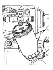
Change the fuel filter. Pump fuel and vent the system. See "Venting the fuel system". Check the fuel hoses as well as the complete fuel system for leakages. If an extra fuel filter is fitted, this filter cartridge must also be changed.
