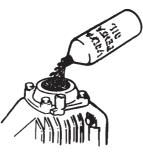
Then reinsert the plug and fill up with oil. Make sure that the oil level is between the maximum and minimum levels indicated on the dipstick. Note: do not exceed the maximum level. See "Technical Data" for type and volume of oil to be used.
