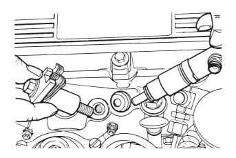
Checking the fuel injectors. All work on the engine fuel injectors must be carried out by an authorized dealer. Check the opening pressure, spray pattern and also check for leakage **every 600 hours of operation.**
