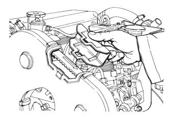
Checking the overhead camshaft drive belt. The toothed drive belt which drives the camshaft should be checked and adjusted by an authorized workshop.
