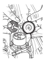
Clean the feed pump filter. Remove the cover and remove the filter.
