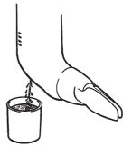
Change the oil in the S-drive. Remove the dipstick. Remove the plug under the propeller gear housing and allow the oil to run out.
