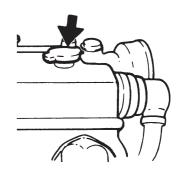
Fill-up the freshwater system to the correct level. Fillup through the filler-hole on top of the heat exchanger with a 50% mixture of freshwater and rust-proofing ethylene glycol or additive.
