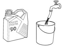
Mix a 50% mixture of fresh water and corrosion-protective anti-freeze.
